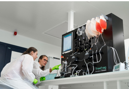
Automated closed system for industrial scale stem cell encapsulation
